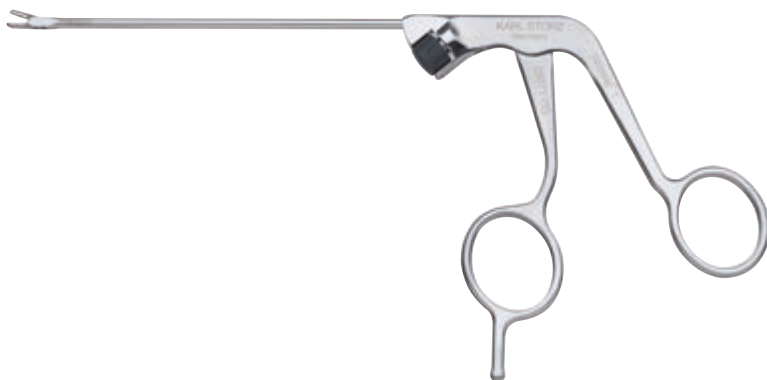
28572CG SILGRASP® PRO Cartilage Grasping Forceps , spoon-shaped jaws, straight jaws, sheath diameter 2.8 mm, straight, handle with cleaning connector, working length 8.5 cm
