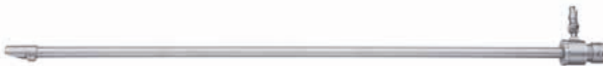
66490 CS Irrigation Sheath , distal irrigation hole with diameter 1.5 mm, irrigation connector with 360° rotating stopcock, 340° rotating light connection, working length 440 mm, for use with Dental Telescope 66490 CF
