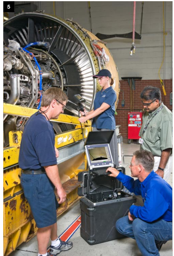
5. Inspectors can use a two-point laser measurement mode
