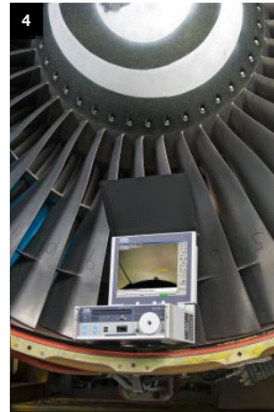
5. Inspectors can use a two-point laser measurement mode
