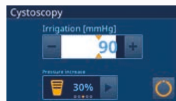
Pressure-controlled irrigation "Cystoscopy" active with activated boost function
