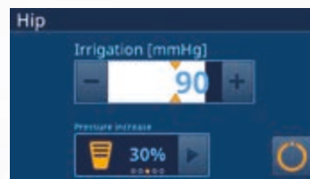
Pressure-controlled irrigation "Hip" active with activated boost function
